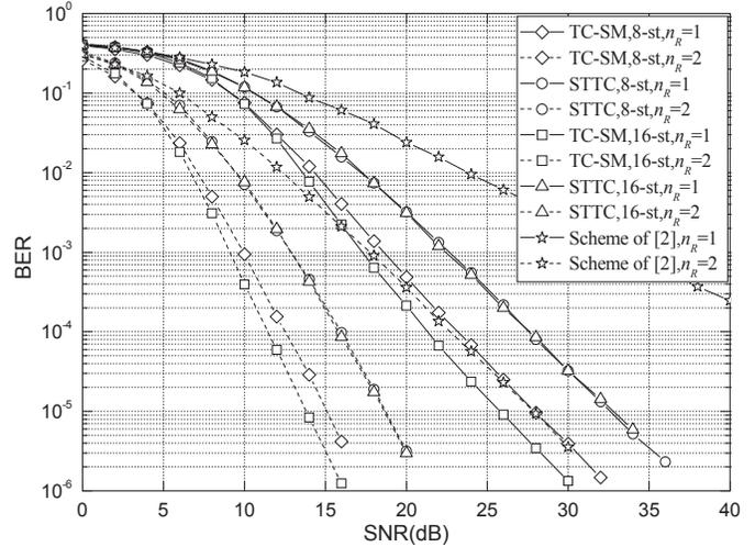
Fig. 4. BER performance for 8- and 16-state TC-SM and STTC schemes with the system of [2] at 3 bits/s/Hz
