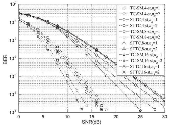
Fig. 3. BER performance for 4-,8- and 16-state TC-SM and STTC schemes at 2 bits/s/Hz
