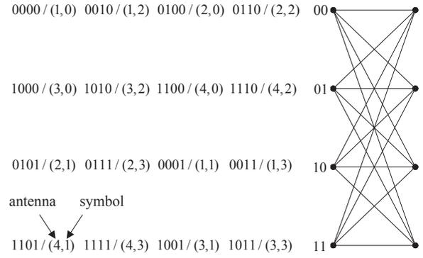
Fig. 2. Trellis diagram of the TC-SM scheme with  $R = 2/4$  trellis encoder, four transmit antennas and QPSK,  $k = 2$  bits/s/Hz.
