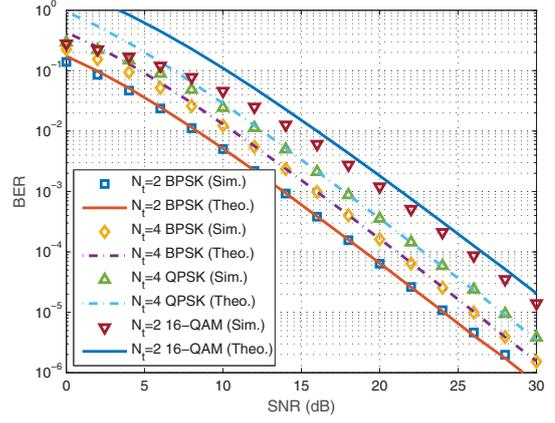
Fig. 3. BER performance of cooperative SM system with DF relaying for different number of transmit antennas and different modulations. Note that  $N_t^S = N_t^R = N_t$  and  $N_r^R = N_r^D = 2$ .
