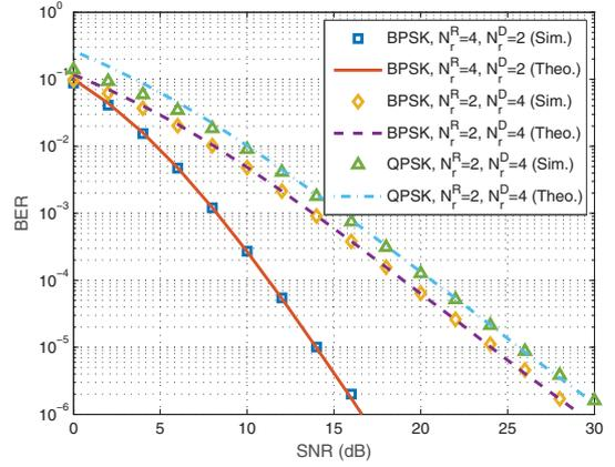
Fig. 4. BER performance of cooperative SM system with DF relaying for  $N_t^S = N_t^R = N_t = 2$ , different modulation orders with respect to different number of receive antennas at R and D.
