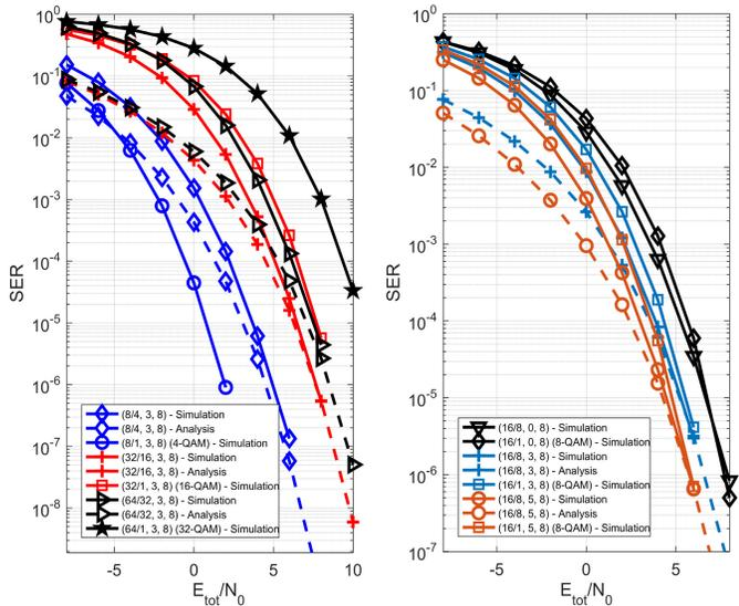
Fig. 3. SER performance comparison of the SSK system  $(N_t/N_s, K, N_r)$  with conventional cooperative MIMO system  $(N_t/1, K, N_r)(Q\text{-QAM})$  for  $N_t \in \{8, 16, 32, 64\}$ ,  $N_s, Q \in \{4, 8, 16, 32\}$ ,  $K \in \{0, 3, 5\}$ ,  $N_r = 8$ .
