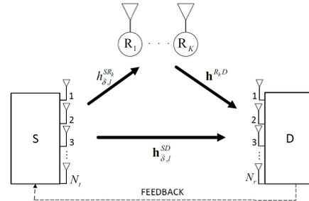
Fig. 1. System model of the SSK with cooperative relays and TAS.
