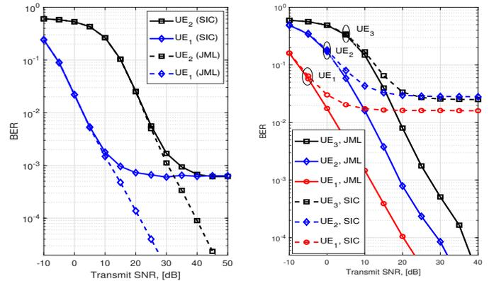
(a) JML vs SIC for  $L = 2$  case. (b) JML vs SIC for  $L = 3$  case.
