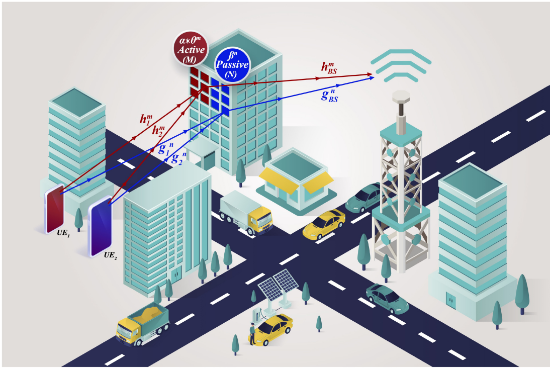
Fig. 1. Proposed over-the-air uplink-NOMA system model for K = 2 users.
